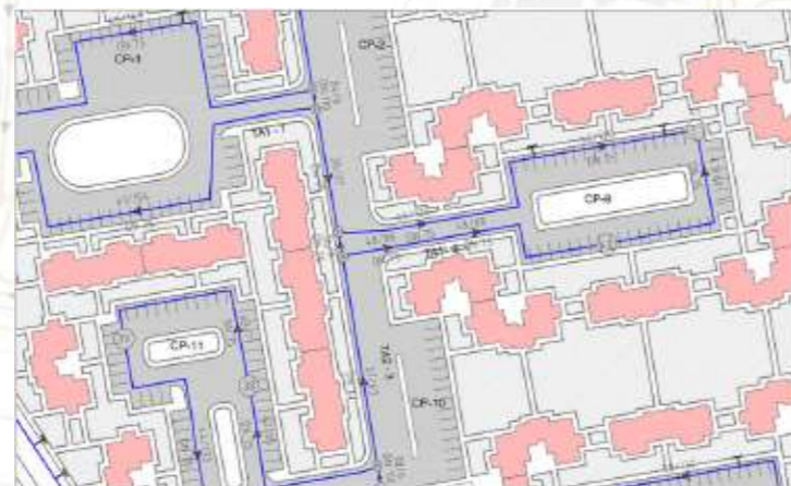
Water Distribution System Model
